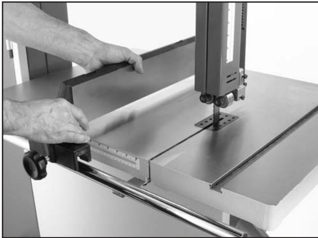
Figure 11. Installing fence onto rail.
